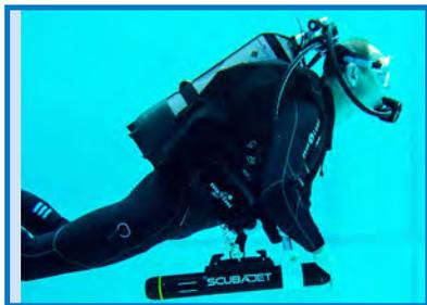
batteries by air. Much smaller, the novel hand-held Scubajet uses jet-power instead of a propeller. Weighing just 6.6 pounds ((3kg), the Austrian-made device generates 44 pounds (20kg)
