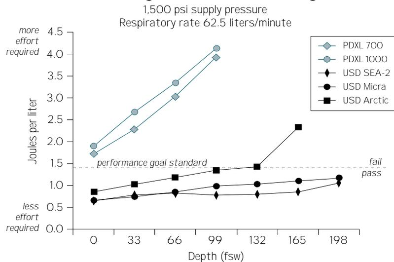
NEDU test results for Performance Diver regulators compared with three USD regulators, including one coldwater regulator
